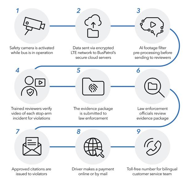
The data relating to the incident and violation is sent via an encrypted LTE network to a secure cloud system, where it is filtered by artificial intelligence (AI) software before being reviewed by a trained safety specialist.
